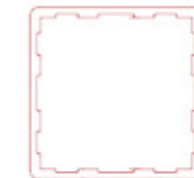
120x120mm Post ( The 120x120mm Post is supplied in conjunction with the Base plate to fix onto a cast concrete footing )
