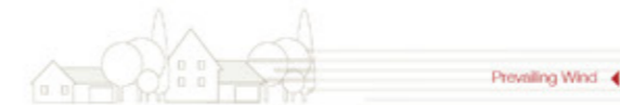
REGION A - N2 (W33), REGION B - N3 (W41) AND REGION C - C2 (W50) Structures built adjacent to an oval or large vacant lot subject to prevailing winds.
