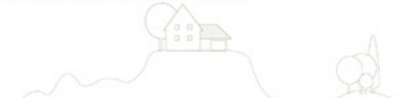
REGION A - N4 (W50) REGION B - N5 (W60) AND REGION C - C4 (W70) Extremely severe - Isolated building on the crest of a hill
