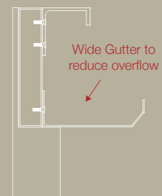
B Support Beam, Stile and Gutter
