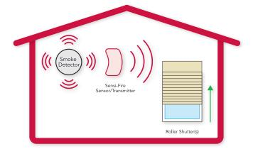
Installation Requirements: The Sensi-Fire Wireless receiver/ transmitter must be positioned within 500mm of a working smoke detector that meets Australian Standards.
