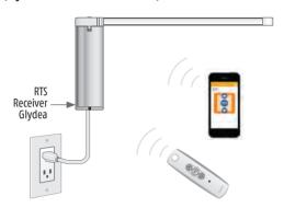
Group and individual control with 4 channel Telis RTS, DecoFlex WireFree™ RTS wall switch and the myLink WiFi to RTS interface. (Glydea® DCT motors + RTS receivers)
