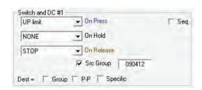
Displayed button configuration will raise the shade on Press, and on Release, the shade will stop at it's current position.
