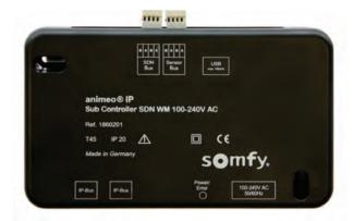
The **animeo IP Sub Controller** expands the system's capacity beyond the initial 200 motors supported by the animeo IP Building Controller. Each additional Sub Controller supports 200 motors.
