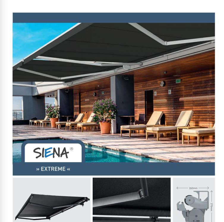
With built-in 8-link stainless steel chain technology and heavy-duty internal spring arms as standard, wide spans are no problems with this supersized solution. Widths up to 15m with 4m projections, installer pitch control options from 0-45°, and front rail and extruded pelmet options available, makes the Extreme the ultimate in design performance.
