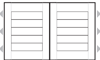
CO - JOINED PANELS Separate panels joined with hinges so they slide as one.
